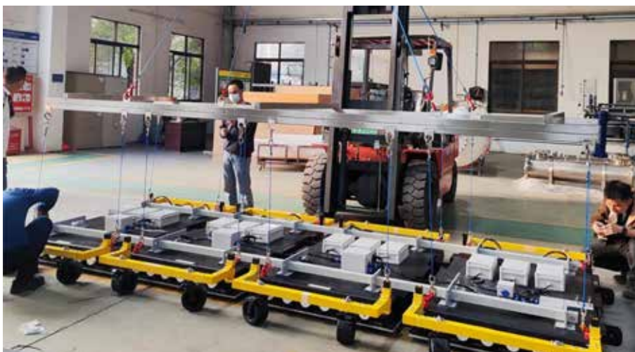
The equipment before shipment to New Zealand – showing four trolleys carrying the UV-C lights linked in a 'train'. Photo: Advanced Aquarium Technologies Ltd.
