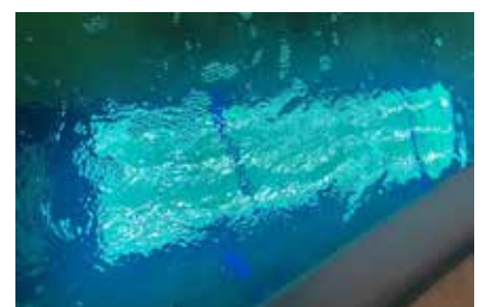
Ensuring the UV-C bulbs are waterproof. Photo: Advanced Aquarium Technologies Ltd.
