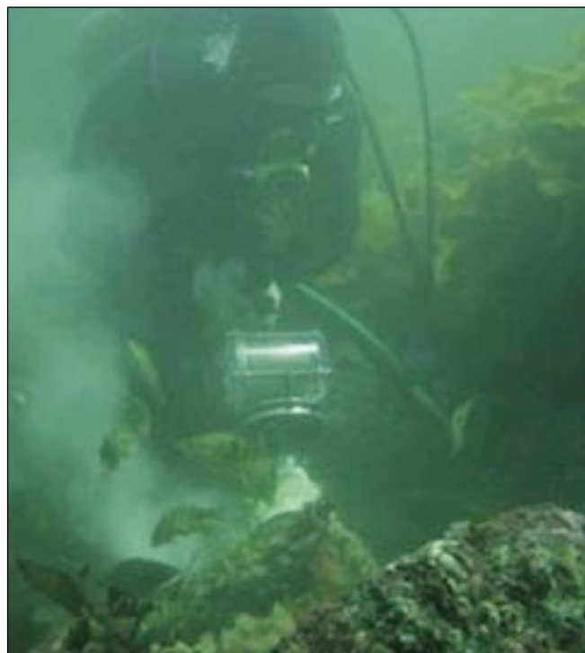
Diver using the steam subsurface steriliser developed by DOC.
