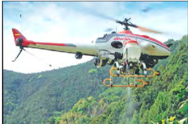
For those hard-to-get weeds: The Yamaha Rmax G/Type 11 unmanned helicopter can carry 28k payload.
